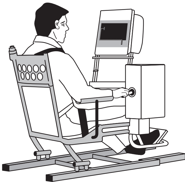
FIG. 1. Subject seated in the experimental setup. The virtual scene was presented on the screen in front of the subject. To manipulate the ROBOTOP joystick with the right hand, subjects rested their forearm in a plastic trough that restricted all movements of the arm except those at the wrist.
