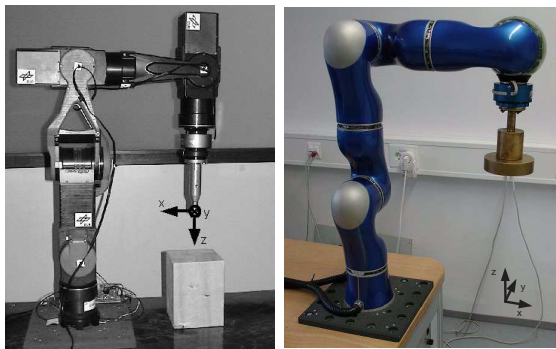
Fig. 6. Initial configuration of the DLR lightweight robots (LWR-II left, LWR-III right) for the experiments.
