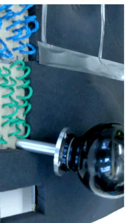
robot adapts geometry *and impedance* to interact with unknown surface characteristics
